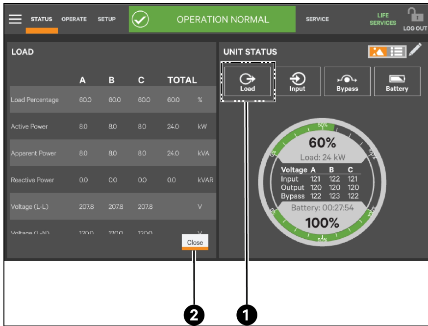
Figure 2.9 UNIT STATUS Pane—Load Details; Graphic Display
