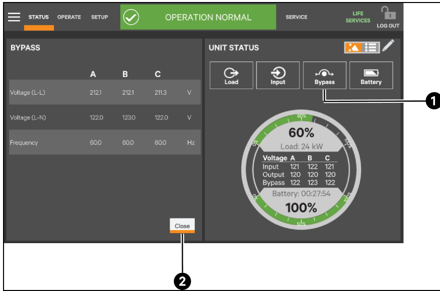
Figure 2.11 UNIT STATUS Pane—Bypass Details; Graphic Display
