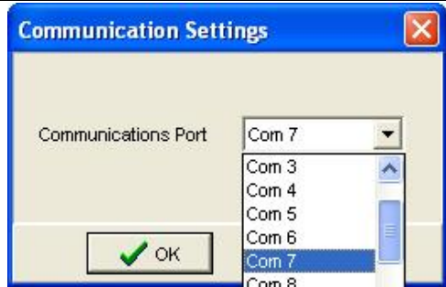
Figure 365. Communications Settings Com Port BAS Software
