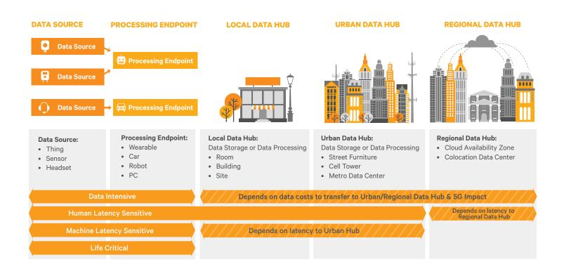
The metro hub leverages the existing telco infrastructure to support the local hub with longer-term data storage and more robust processing capabilities. The regional hub is likely to be a cloud data center operating in the same region as the local hub.
