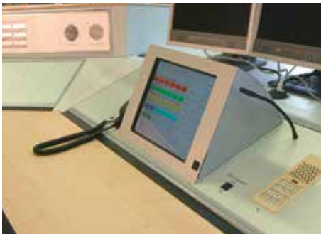
Tilt adjustment for built-in monitors
