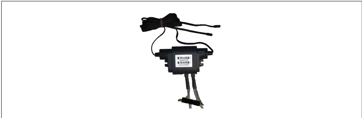
Figure 13.8 CANbus and ground connection on 2T sensor
