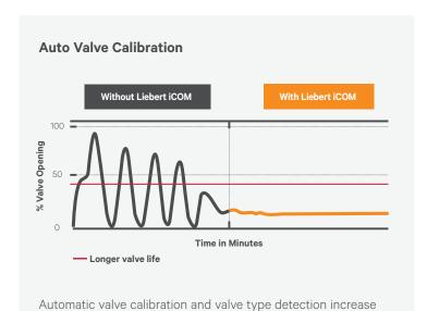
valve life expectancy by only moving the valve in increments
