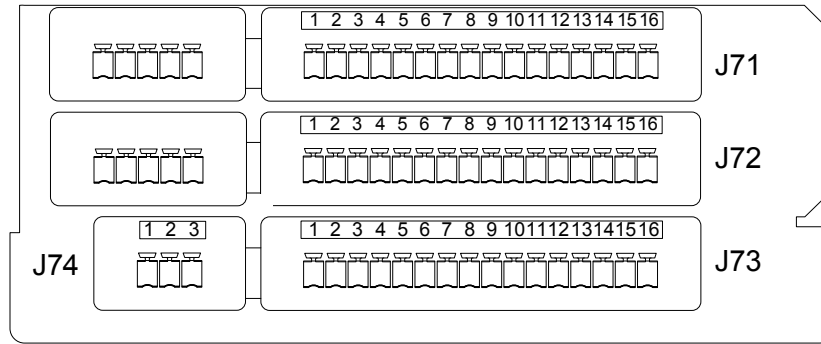
Figure 12 Control wiring, Programmable Relay Board
